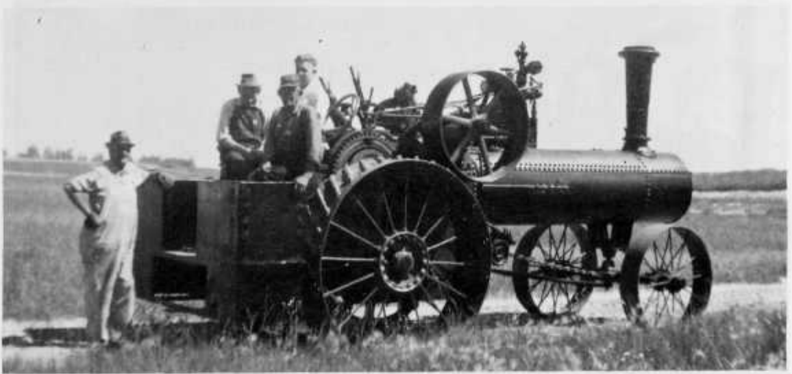
Restored 1912 model of 20-60 Case Steamer, engine no. 28286. The engine was purchased in 1957 from John Midboe of Fosston, Minnesota. The engine has been completely rebuilt over a period of five years, putting in a new set of flues, cleaning and painting and making a set of coal bunkers.
