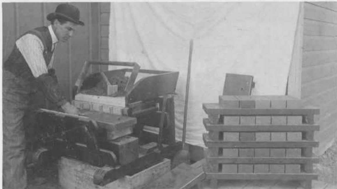
This cement brick machine was constructed and used by Charles F. Culp in 1906-07. A patent was allowed for the machine following application by Culp.
